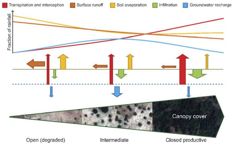
Figure 5.2. A conceptual drawing of the “optimum tree cover”-theory proposing that groundwater recharge will be greatest under an intermediate tree cover (Ilstedt et al., 2016).
